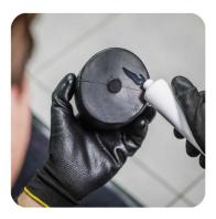
Warning: Lubricate also the lateral surfaces of the
