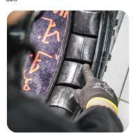
In intermediate configurations it will be normal to have empty spaces between one insert and another (about 1-2 cm / 0,4-0,7 inch)
