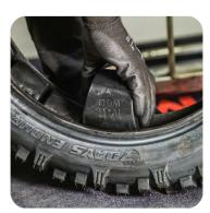
Insert the Balls inside the tire
